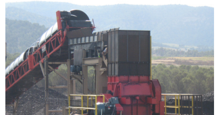
Achieve a 6:1 reduction ratio in the primary stage and a 4:1 in the secondary.
